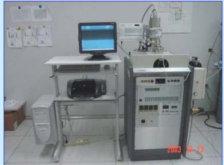
Internal Vapor Analyzer System
